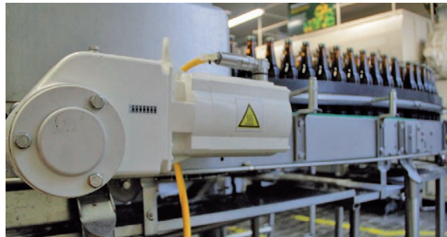
Motor-prevodovka Danfoss VLT® OneGearDrive
